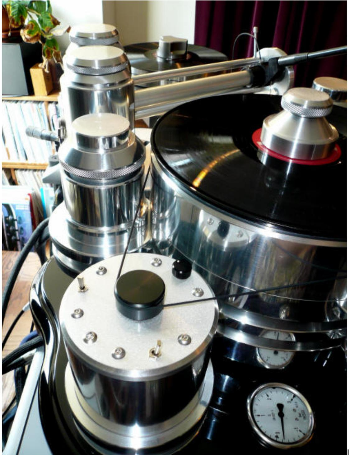
in the meantime the two vacuum rings on the platter, one on the outer rim and the other halfway in, grab hold of the record. You'll see even warped LPs flatten after the vacuum clamps it down.
