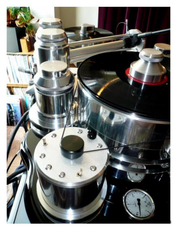
n the meantime the two vacuum rings on the platter, one on the outer rim and the other halfway in, grab hold of the record. You'll see even warped LPs flatten after the vacuum clamps it down.
